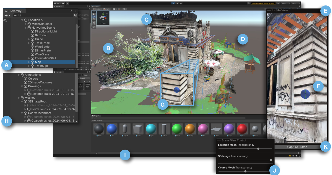
Figure 6: Ex-situ user interface of CoCREATAR. (A) All objects under NetworkedScene are automatically synchronized between ex-situ and in-situ users; (B) 3D Snapshots captured by the in-situ user; (C) The location mesh of Location A; (D) Coarse Mesh captured by the in-situ user; (E) Live feed of the in-situ user’s screen, including AR content; (F) The 3D Cursor of the ex-situ user, projected into world space; (G) Close-up of the 3D Cursor of the ex-situ user as seen in the scene view; (H) List of annotations and spatial captures, persistently saved in the scene for later review; (I) Sample assets that can be added to the scene at runtime.
